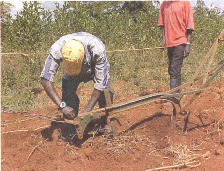
Plate 3: Adjusting furrow depth by shifting the hitching point
