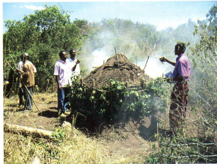
Traditional kilns where recovery is less than 20% should be avoided
